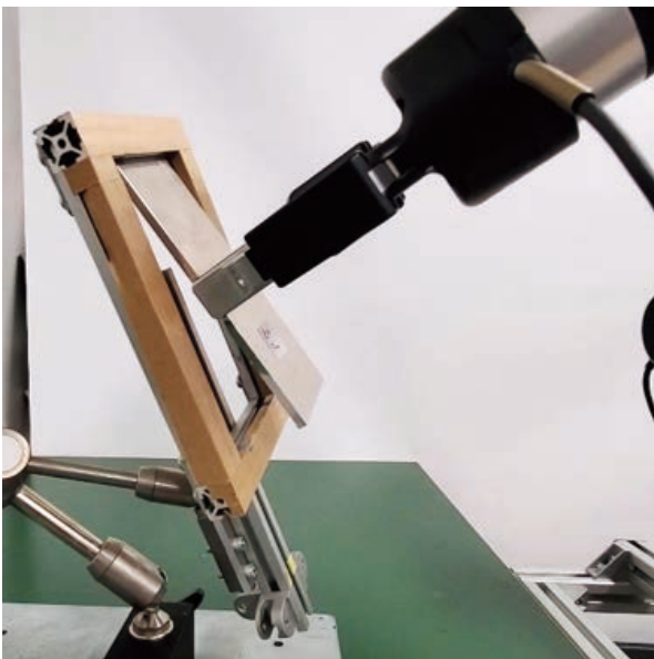
Fig.3. Sash insertion task as a robotic assembly.
